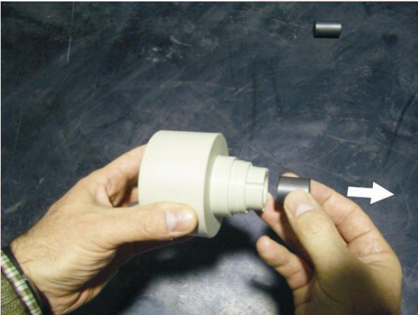
13) Remove front and rear internal magnet bushings and check status.
