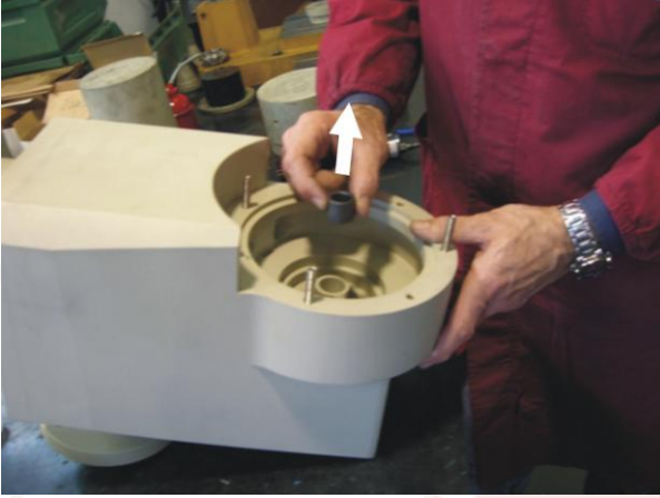
13) Remove front and rear internal magnet bushings and check status.
