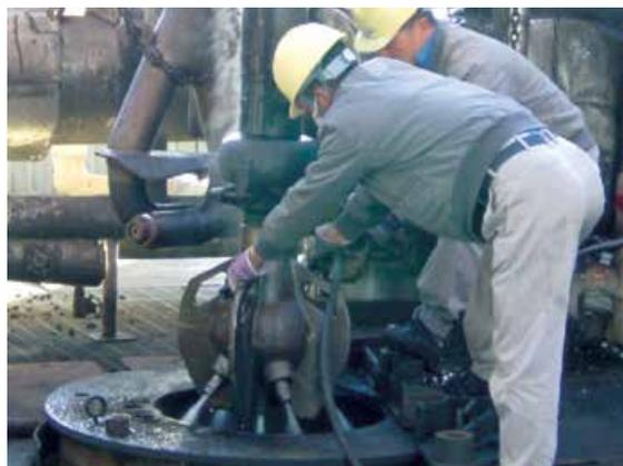
*With manual mode shifting, personnel may be exposed to hazards at the drumhead.*
