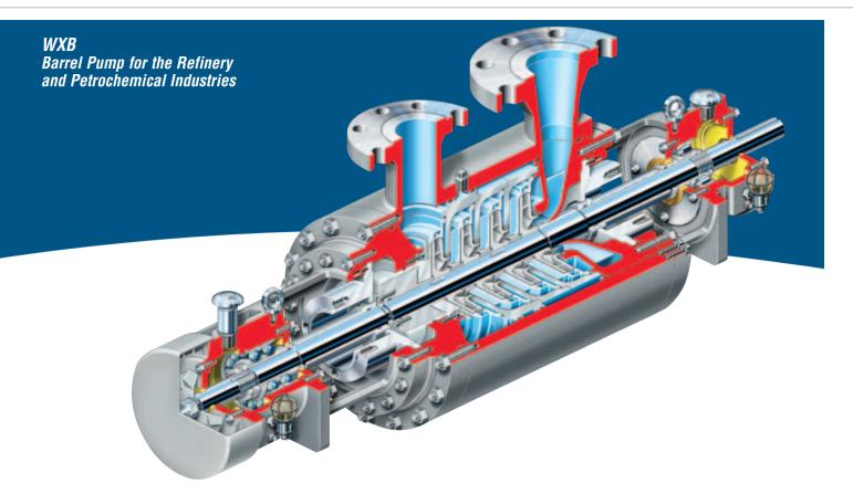
The WXB is an API style barrel pump that offers maintenance-friendly features such as a cartridge design and renewable wear rings. It is designed for users looking for a cost-effective high-pressure process pump with the safety attributes of a double-case design.
