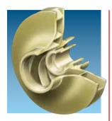
Precision Cast Closed Impeller is statically and hydraulically balanced to reduce power consumption. The impeller is keyed to shaft to provide positive drive and eliminate impeller spin-off. Balancing holes through the impeller hub minimize axial thrust and seal chamber pressure.
