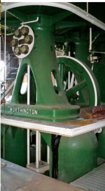
Steam-driven water pump installed in the late 1800s
