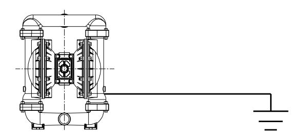
To reduce the risk of static electrical sparking, this pump must be grounded. Check the local electrical code for detailed grounding instruction and the type of equipment required, or in the absence of local codes, an industry or nationally recognized code having juristiction over specific installations.
