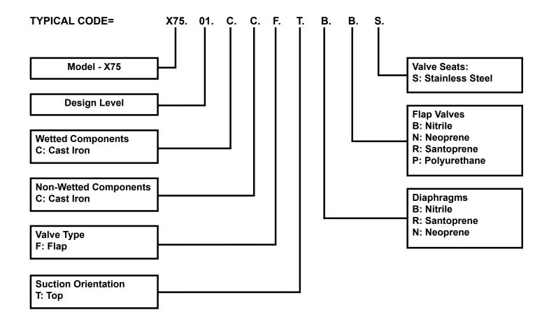
Maximum delivery: 988 ltrs/min Max. working pressure: 8.6 bar Max. solid particle size: 75mm
