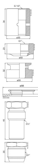
Hygienic welding adapter suitable for tank installation of: TE67Ox4xxxxxx and TE67Gx4xxxxxx Item number: TE67N000000005, TE67N000000006, TE67N000000012, TE67N000000013
