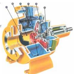
If for some reason, air penetrates into the suction pipe and the pump stops pumping, the priming process starts again and described above, and continues until normal pumping has been resumed
