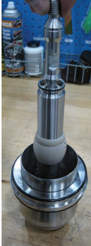
14. Tighten. Use a 13mm and 16mm wrench. Torque 20Nm.
