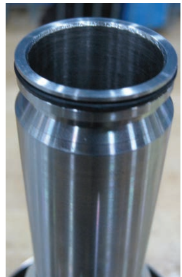
5. Mount o-ring on upper plug.
