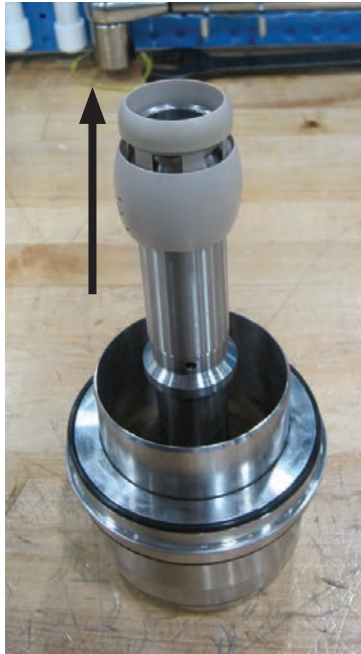
13. Remove lock ring and rotating nozzle by pulling upwards.
