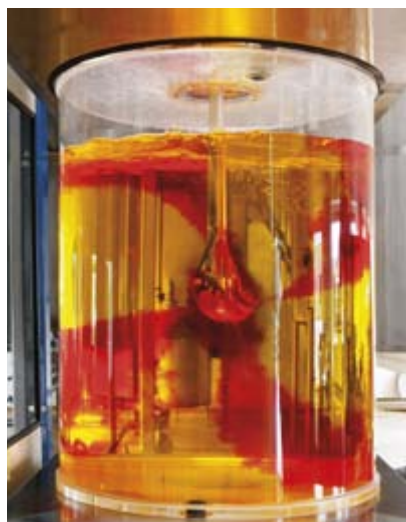
Iso-Mix rotary jet mixers inject fluid, gas or powder through rotating jet nozzles – without causing the liquid to rotate.
